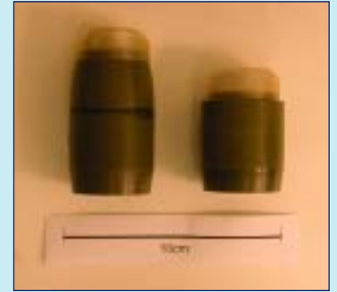
Medium calibre variants (of different mass and aerodynamic properties) of 37 mm DIP concepts, showing the carrier body and irritant payload in the nose, within a frangible cap.
